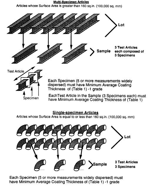
All Test Articles (Specimens) Together must have Minumum Average Coating Thickness of (Table 1)
