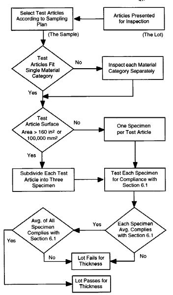
FIG. 3 Coating Thickness Inspection Steps
